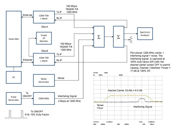
Figure 1 Test Setup for Interference Testing
